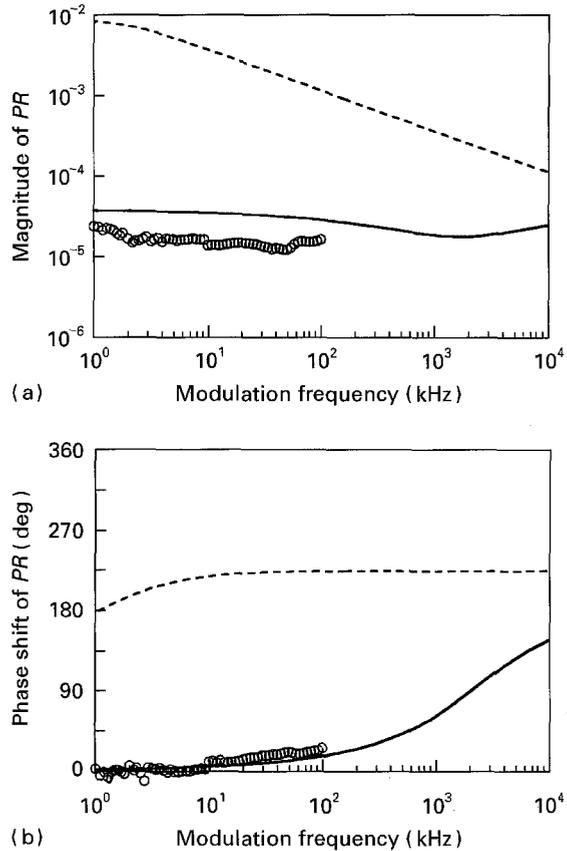
Figure 4 (a) Variation of the magnitude, and (b) phase of the calculated and measured photoreflectance with the modulation frequency in a silicon wafer. (---) One-dimensional analysis, (—) three-dimensional analysis. (O) Experimental data (effective beam radius =  $2 \mu\text{m}$ ,  $D = 20 \text{ cm}^2 \text{ s}^{-1}$ ,  $\tau = 100 \mu\text{m}$ ).
