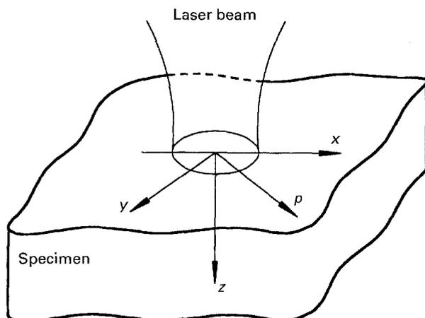
Figure 1 The coordinate system for the calculation of the photoreflectance.
