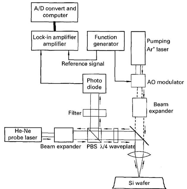
Figure 3 A schematic diagram of the experimental equipment for the measurement of photoreflectance.
