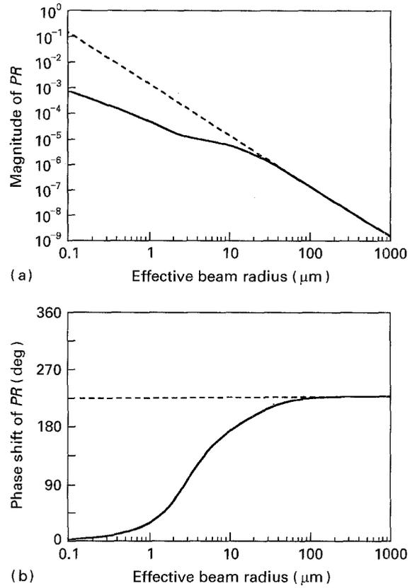
Figure 2 (a) Variation of the magnitude, and (b) phase of the calculated photorefectance with the effective beam radius in a silicon wafer. (---) one-dimensional analysis, (—) three-dimensional analysis. Modulation frequency = 1 MHz,  $D = 20 \text{ cm}^2 \text{ s}^{-1}$ ,  $\tau = 100 \mu\text{m}$ .
